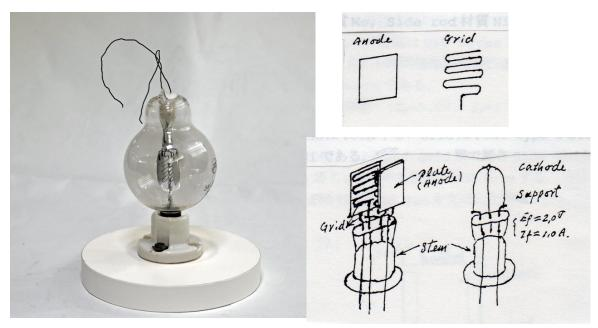
Note: Filament is a reversed-V shape with a center supporting rod ---- Ed..
